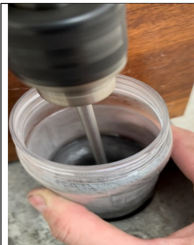
Figure 1: Pre-dispersion of NGDA (Tylose_NG)
